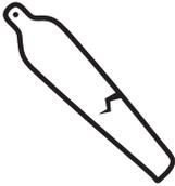
Check your propellers for damage before flying
