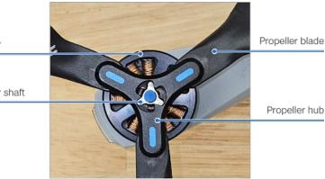
Step 3 - Apply firm opposite torsion between the propeller hub and the motor in both directions without pressing down
