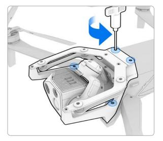
Step 3 - Remove the sensor package
