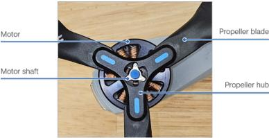
**Step 3** - Apply firm opposite torsion between the propeller hub and the motor in both directions without pressing down
