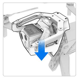
Step 5 - Press sensor package into place
