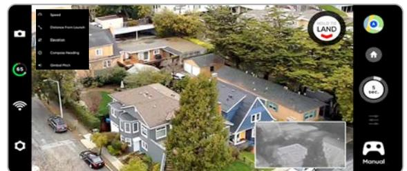
**PIP** (X2D Color/Thermal only) - live feed of the thermal camera. Tap on the PIP to toggle between viewing the thermal camera feed full screen and the color camera feed full screen.
