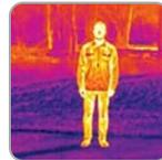
**Ironbow** - uses color to display heat distribution and thermal anomalies. Warmer objects are presented in lighter colors and colder objects in darker colors.
