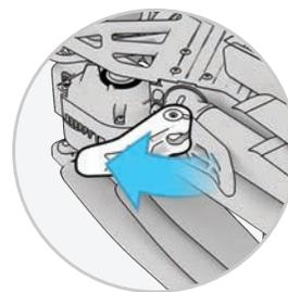
**Step 3** - Return the 4 arm clamps to the locked position
