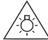
Do not stare directly into the Spotlight attachment or a sensor package flashlight at any distance range for any period of time as it may cause serious eye injuries.
