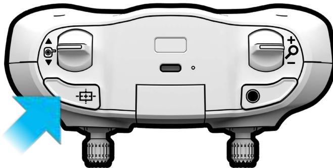
The **left shoulder button** activates the **Boost** feature. **Boost** allows you to instantly increase the speed of your movement while holding down the **left shoulder button**. To stop using **Boost**, release the **left shoulder button**. Use **Boost** to quickly fly between points of interest without having to manually increase the control sensitivity in the Skydio app settings.
