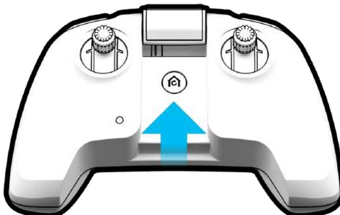
When Skydio 2 is in flight, tapping on the **Return Button** commands Skydio 2 to return to its launch location. If you have set a home point on the map, pressing the **Return Button** will command Skydio 2 to return to the Home Point instead of the launch location. You may press the **Return Button** again to stop returning.
