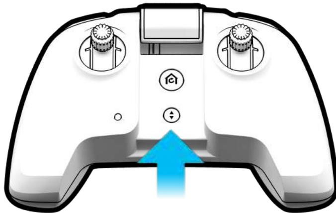
You may end your flight by using the **Land button**. When landing Skydio 2, ensure the drone is situated over a safe landing spot that is flat, clear of debris and not overhead of any people or animals. When you are ready to start landing, hold the **Land button**.
