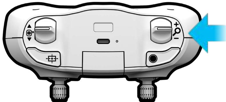
The **right paddle** allows you to zoom in and out of the current view by commanding Skydio 2 to fly directly forwards or backwards in relation to the current camera pitch. When used in combination with the gimbal control and **Boost** feature, this allows for dramatic FPV style flying.
