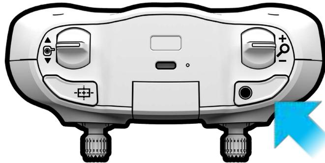
The **right shoulder button** acts as your shutter. The shutter button allows you to capture a photo while in photo capture mode or start and stop recording when in manual video capture mode. The right shoulder button does not have any effect while in auto video capture mode.
