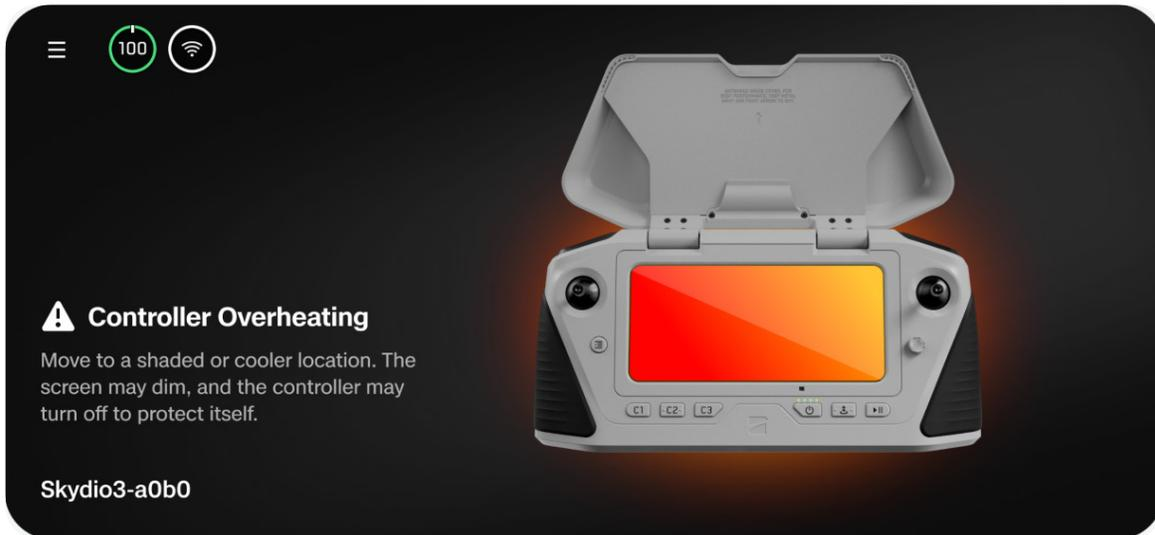
To mitigate overheating and reduce the risk of lost connection during flight, the controller will issue two alerts and provide guidance to the operator.
