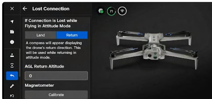
After 5 seconds of inactivity in Attitude Mode (i.e. the joysticks are centered and not touched in a neutral position and not engaged), Skydio X10D will automatically initiate an emergency landing and descend autonomously. An alert notification will display that Skydio X10D is initiating an emergency landing. If you input any joystick command while the drone is emergency landing, it will stop descending landing and you can continue to fly in Attitude Mode.
