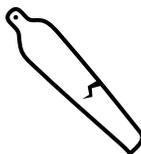
Check your propeller blades for damage before each flight.
