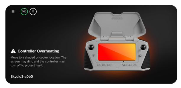
To mitigate overheating and reduce the risk of lost connection during flight, the controller will issue two alerts and provide guidance to the operator.
