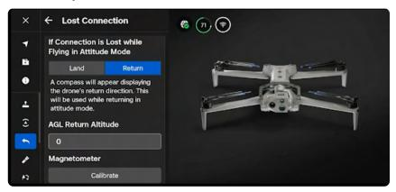
After 5 seconds of inactivity in Attitude Mode (i.e. the joysticks are centered and not touched in a neutral position and not engaged), Skydio X10D will automatically initiate an emergency landing and descend autonomously. An alert notification will display that Skydio X10D is initiating an emergency landing. If you input any joystick command while the drone is emergency landing, it will stop descending landing and you can continue to fly in Attitude Mode.
