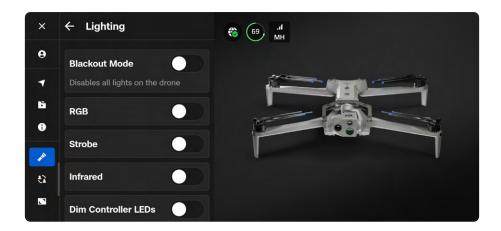
**Blackout Mode** - Enabling Blackout Mode will turn off all visible and IR light sources on the vehicle, disable the light toggles, and dim the controller lights. Setting Blackout Mode will persist across flights and power cycles.
